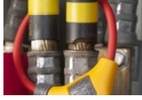
flexible current probes are used when conductors are too large for a clamp
