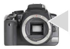
When Lisa opened the box firstly she found the DSLR camera body. DSLR stands for a digital single-lens reflex and a 'body' is the main camera part without a lens attached. Then there was a lot of other little bits and pieces that came in the box.
